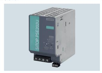
The SITOP PSE202U redundancy modules are the optimal extension for all 24 V power supplies to ensure additional protection from failure of the 24 V supply. The redundancy module continuously monitors the power supply units and, in the event that one unit fails, the other unit automatically takes over the 24 V power supply. Additionally, a signal is sent via a signaling contact that can be evaluated by a controller, PC, or control system.
