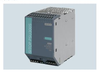
The three-phase SITOP smart are the universal and powerful standard power supplies for machinery and plant engineering. Despite their compact design, they offer an excellent overload response: Thanks to an extra power of 150 %, loads with high power consumption can be connected without any problems and the permanent overload capability of 120% offers power reserves in case of expansions.
