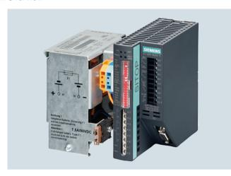
By combining a DC UPS module with at least one 24 V battery module and a SITOP power supply unit, longer power failures can be bridged without any interruption. Even if a greater buffering current is required, the DC UPS with maintenance-free lead battery provides optimum safety. It spans power failures up to several hours long and delivers up to 40 A.
