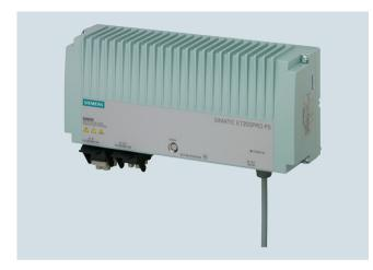
The SIMATIC ET200pro PS power supply unit with degree of protection IP67 is used as the electronics/encoder supply and load voltage supply of the new SIMATIC ET 200pro distributed I/O system for use close to the machine without a cabinet. With a signaling contact for "24 V OK" and "Overtemperature", as well as a second plug-in connector for input voltage loop-through.
