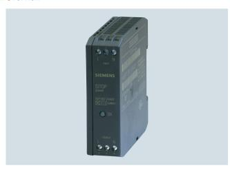
The SITOP inrush current limiter is used to reliably reduce the starting currents that are caused, for example, by transformers or with pulse-controlled power supplies by the rectifier circuit on the input side with capacitor charging.
