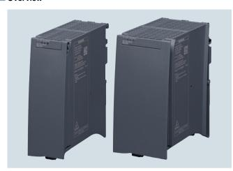
The design and functionality of the SIMATIC PM 1507 single-phase load power supply (PM = power module) with automatic range selection of the input voltage makes it an optimal match to the SIMATIC S7-1500 PLC. It supplies the S7-1500 system components such as CPU, system power supply (PS), I/O circuits of the input and output modules and, if necessary, the sensors and actuators with 24 V DC.
