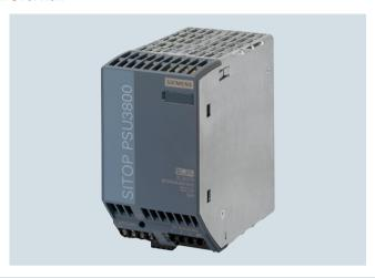
SITOP PSU3800 3-phase power supplies (24 V DC/17 A and 30 A) are suitable for battery charging, thanks to their constant-current characteristic. For other applications the output characteristic can also be switched to latching shutdown. The three-phase, wide-range input enables them to be used worldwide. The slim design requires little space on the DIN rail. Installation gaps are not required.
