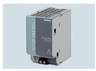
The SITOP PSE201U buffer module bypasses short-term power failures lasting a few seconds and can be used with all 24 V power supplies of the SITOP smart or SITOP modular product lines. The buffer module is equipped with maintenance-free capacitors and automatically takes over the 24 V power supply in case of a power supply failure.
