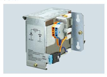
Maintenance-free battery modules with 1.2 Ah up to 12 Ah (lead-gel accumulator) for ambient temperatures from 0 to +40 °C as well as high-temperature battery module with 2.5 Ah (pure-lead accumulator) for ambient temperatures of -40 °C to +60 °C. The battery modules are completely prewired with battery retainer and terminals. For longer buffer times, the battery modules can be connected in parallel. Mounting onto standard mounting rail or directly to the wall.
