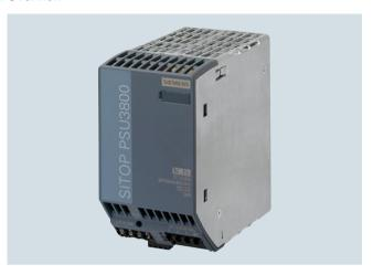
The SITOP PSU3800 3-phase power supplies are suitable for battery charging, thanks to their constant-current characteristic. For other applications, the output characteristic can also be switched to latching shutdown. The three-phase, wide-range input enables them to be used worldwide. The slim design requires little space on the DIN rail. Installation gaps are not required.
