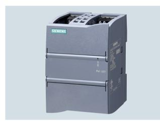
In terms of design and functionality, the SIMATIC PM 1207 single-phase load power supply (PM = power module) with automatic range selection of the input voltage is an optimal match to the SIMATIC S7-1200 PLC. It provides the supply to CPUs with 24 V input as well as to signal modules, and to 24 V loads connected to the modules. Comprehensive certifications, such as UL, ATEX and GL facilitate universal use.
