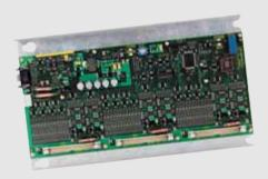
The PP 72/48 I/O module is connected to PROFIBUS DP and provides 72 digital inputs and 48 digital outputs. The 3 plug-in connectors for the inputs and outputs are 50-pole terminal posts for connecting ribbon cables. Terminal strip converters can be used or the direct connection of distribution boards, for example, is possible.
