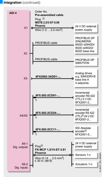
The max. cable lengths depend on the current consumption, power supply and frequency of the encoders (see Manual SINUMERIK and SIMOTION ADI 4).
