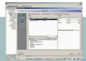
The drive and control configuration is stored in a project. The components and functions used are displayed in a tree
