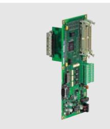
The MCPA module features interfaces for the connection of an analog spindle, the MCP 802D sI machine control panel and terminal strips for additional, high-speed NC inputs and outputs. The MCPA is mounted on the rear side of the PCU of the SINUMERIK 802D sl. The specially provided mounting location is protected by a cover. The installation kit is included in the scope of supply.
